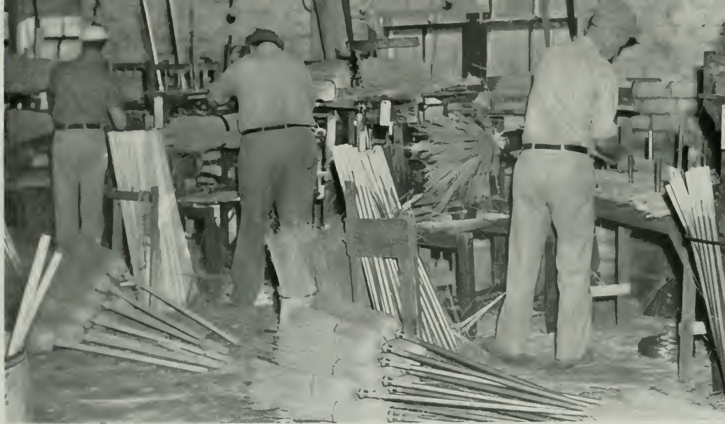
This is the winding operation in making a broom. Man at right is building up broom, using rough corn in center and better fibers on outside. A broom is appraised for its weight, which depends on the knack and feel of the man making it.
