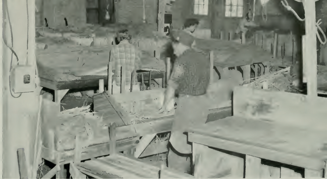
A scene in a broomcorn factory at Arcola; corn is sorted manually as to length, color and texture of fiber. The coarser fibers are used for industrial broomcorn, while the rest goes into house brooms or whisk brooms.
